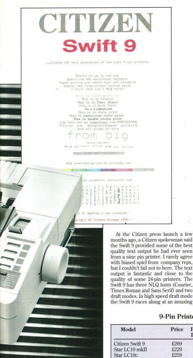
213 characters per second (cps). In standard draft mode the print quality betters and the machine slows to 192 cps. In NLQ it handles 40 cps with easy and relative quietness – 51dB in fact.
